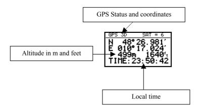
Rotating up/down selector to the right will extend altitude indication with feet reading also. The stop watch is working under following propositions.
